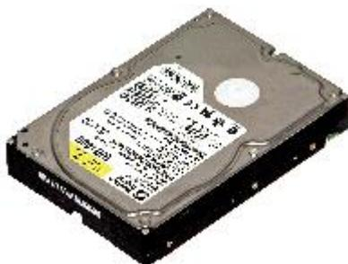
Hard disks are made up of rigid material and are usually a stack of metal disks sealed in a box. The hard disk and the hard disk drive exist together as a unit and is a
