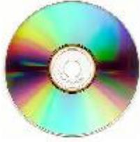
Compact Disk (CD) is portable disk having data storage capacity between 650-700 MB. It can hold large amount of information such as music, full-motion videos, and text etc. CDs can be either read only or read write type.
